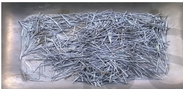
Figure – 2 Sample of Galvanized iron fibres
